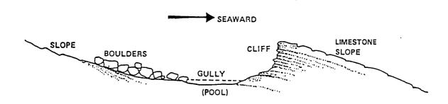
FIGURE 1 . REPRESENTATIVE DIAGRAMMATIC SECTION OF HINKLEY POINT ROCK FORESHORE
